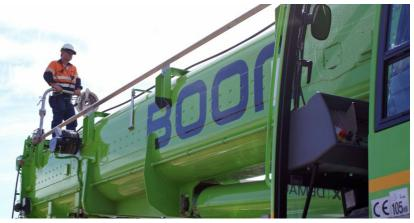
**TRAM** technology utilizes a handhold that moves with the operator (vertically and horizontally) and acts as a moveable anchor point for the restraint harness.
