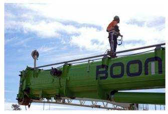
**Site Installed** cranes often have height restrictions for access areas on the top side of the boom, where motors and cable drums are housed. This removes the possibility of hand rails and other such passive safety systems.
